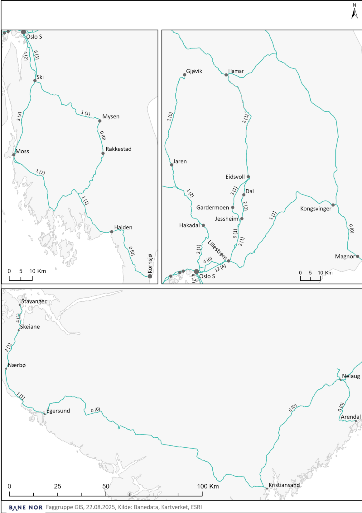
Map 5d Traffic flow on local and regional trains; Number of trains per hour per direction (additions during peak hours)
